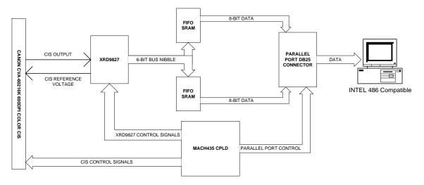
Figure 1. Block Diagram of XRD9827REF
